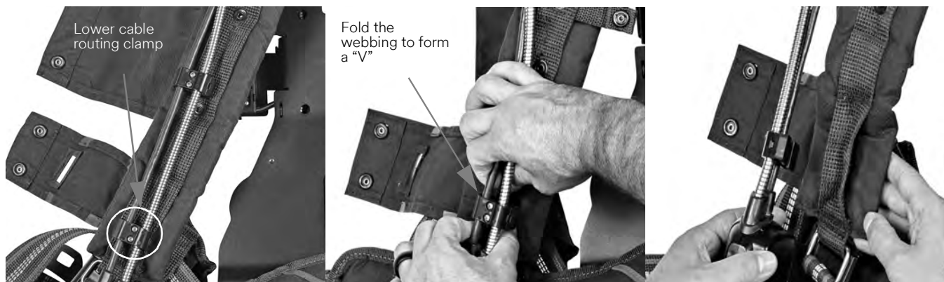
Figure 2-4 Removing the lower cable routing clamp
