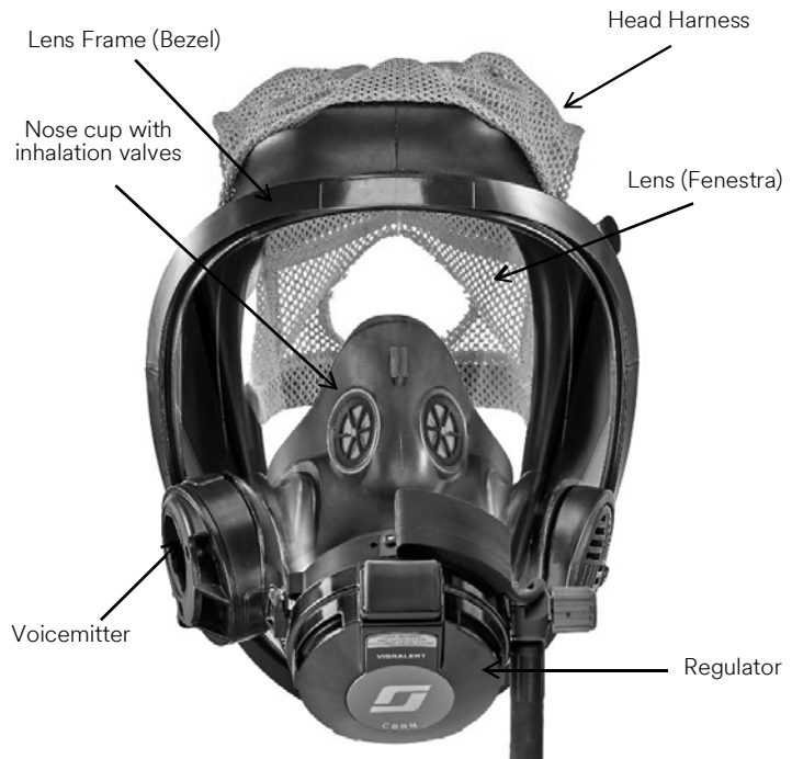
Figure 1-3 Facepiece components (3M™ Scott™ AV-3000 HT Facepiece shown)
