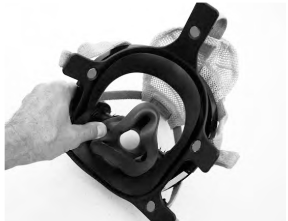
Figure 1-4 Checking the nose cup installation
