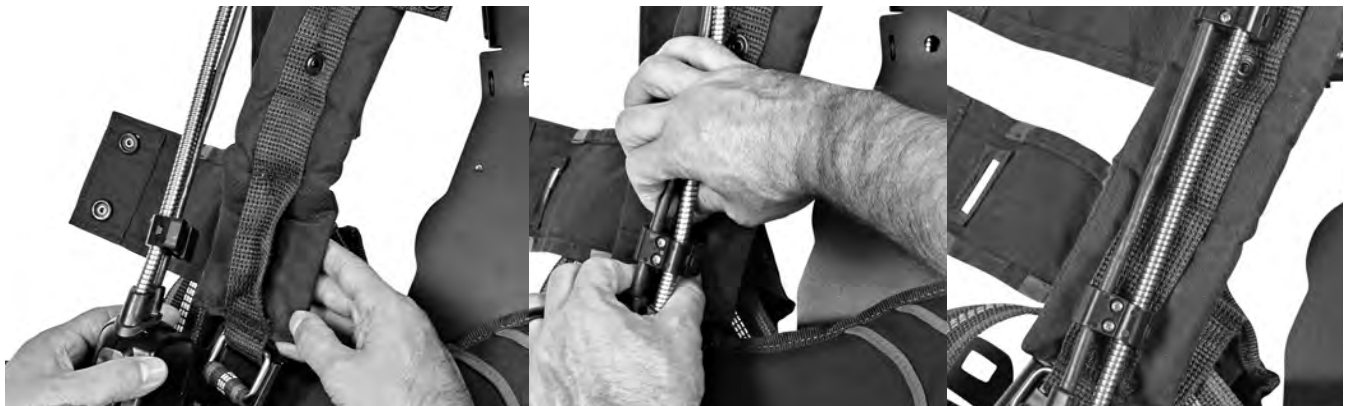
Figure 2-27 Attaching the lower cable routing clamp
