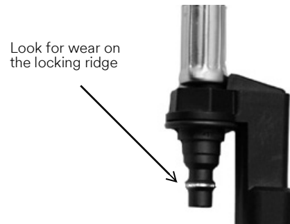
Figure 1-6 Inspecting the male quick-disconnect
