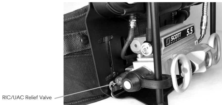
Figure 1-2 Inspecting the RIC/UAC connection
