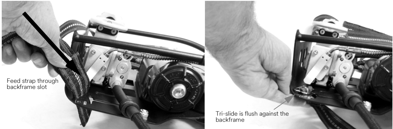
Figure 2-17 Feeding the waist-to-shoulder strap through the backframe slots.
