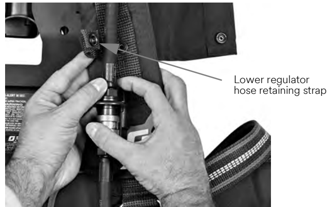
Figure 2-5 Unsnapping the regulator hose retaining strap
