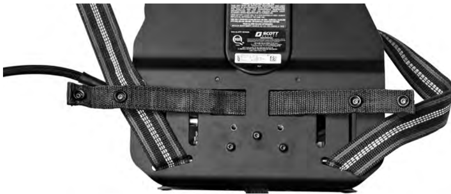
Figure 2-18 Installing the waist pad retaining strap to the backframe
