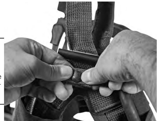
Figure 2-28 Securing the cables and hose
