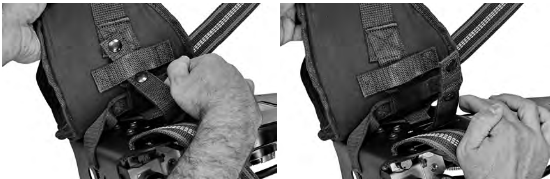
Figure 2-12 Sliding the waist pad retaining strap through the waist pad loop
